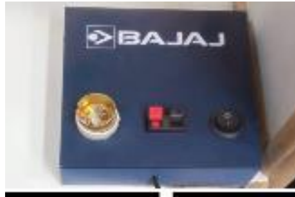
Bulb Tester Unit placement
