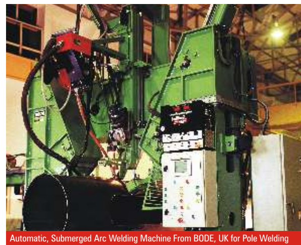
Automatic, Submerged Arc Welding Machine From BODE, UK for Pole Welding
